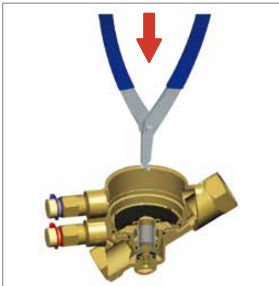
Step 5: Insert the nose pliers through the center of the cartridge
