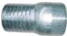
Combination Nipple Standard Thread : NPS, BSP Material : Galvanized Steel, Stainless Steel Working Pressure : 150 psi.
