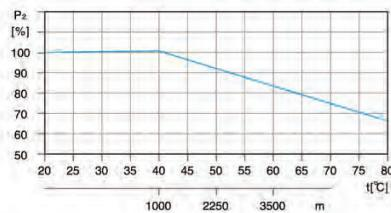
For example, when the pump is installed at altitude of more than 3500 meters above sea level,  $P_2$  will be decreased to 88%. When the ambient temperature is 70°C,  $P_2$  will be decreased to 78%.
