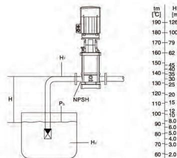
Note: To avoid cavitation, never select a pump with a duty point too far to the right on the NPSH curve.
