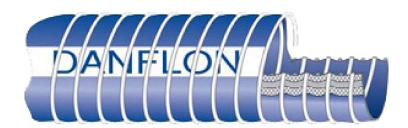
Used Worldwide by many leading companies, these premium quality hoses are lined, as standard, with Ethylene Chloro Tri Fluoro Ethylene (ECTFE). This is a high tech fluropolymer very similar to Poly Tetra Fluoro Ethylene (PTFE) in its broad spectrum chemical resistance but with the advantage of high mechanical strength and low permeability. The inner and outer wires can be galvanised carbon steel or stainless steel 316.
