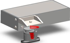
7. When the machine base floats on vibration isolator and is level, tight all the Leveling Bolt + washer.
