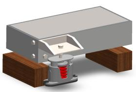
6. Check level of equipment and adjust each vibration isolator so that is the equipment is level. By turning the Leveling Bolt counterclockwise, it will increase the level and turning clockwise will adjust the level down.
