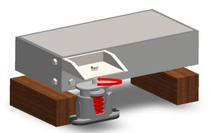
5. Repeat step 4 with each vibration isolator in order until spring is pressed and temporary support is loose enough to be able to removed. (In case some temporary support become loose, stop adjusting the Leveling Bolt of the Vibration Isolator at that point and adjusting the Leveling bolt of vibration isolator in another area instead until all temporary supports are loose enough to be removed.
