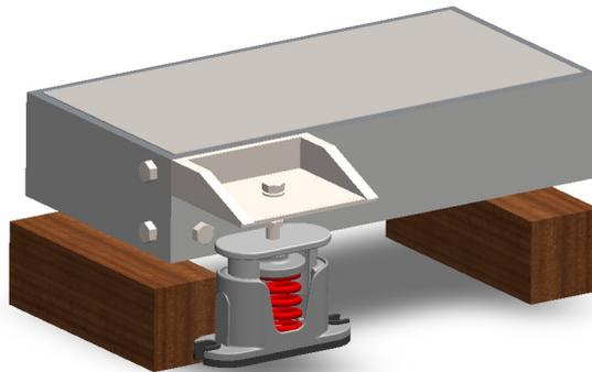
6. Check level of equipment and adjust each vibration isolator so that is the equipment is level. By turning the Leveling Bolt counterclockwise, it will increase the level and turning clockwise will adjust the level down.
