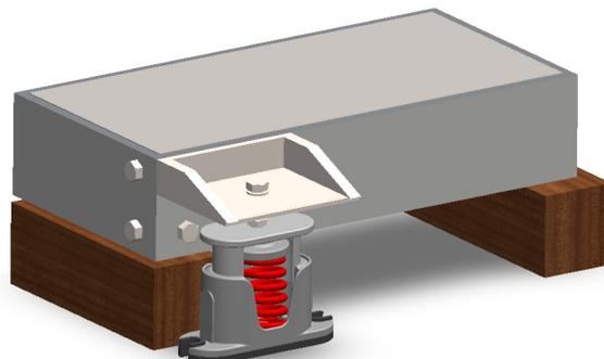
4. Transfer the weight of equipment to spring by turning each Leveling Bolt counterclockwise 2 full turns.
