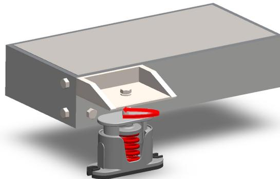
7. When the machine base floats on vibration isolator and is level, tight all the Leveling Bolt + washer.
