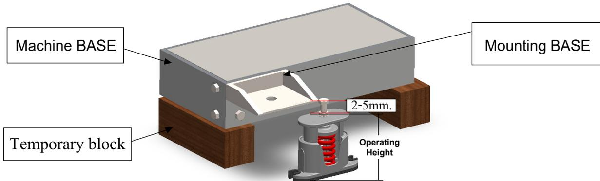
2. Connect the equipment to system and fill the system or add water (Vibration isolator should be at normal operating weight before adjusting the spring).
